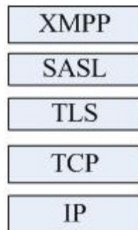
Figure 2: Security layers in XMPP [4].
